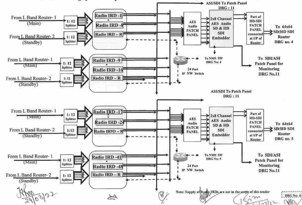
Suggestive Block Schematic for SITC of DD DTH expansion by upgradation of existing four compression chain and monitoring system - Input Base Band-Radio Service (For Stream 4N & 5N)
