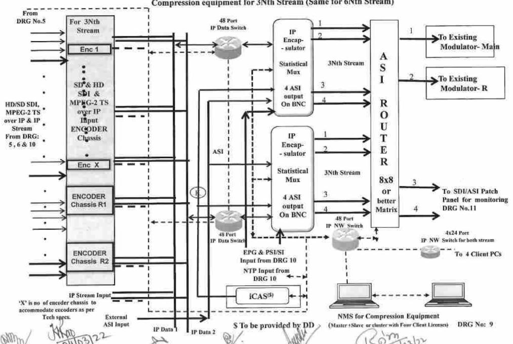
Suggestive Block Schematic for SITC of DD DTH expansion by upgradation of existing four compression chain and monitoring system -Compression equipment (EPG & PSI/SI Generator, NTP Server and IP Input Streaming for Radio Service)
