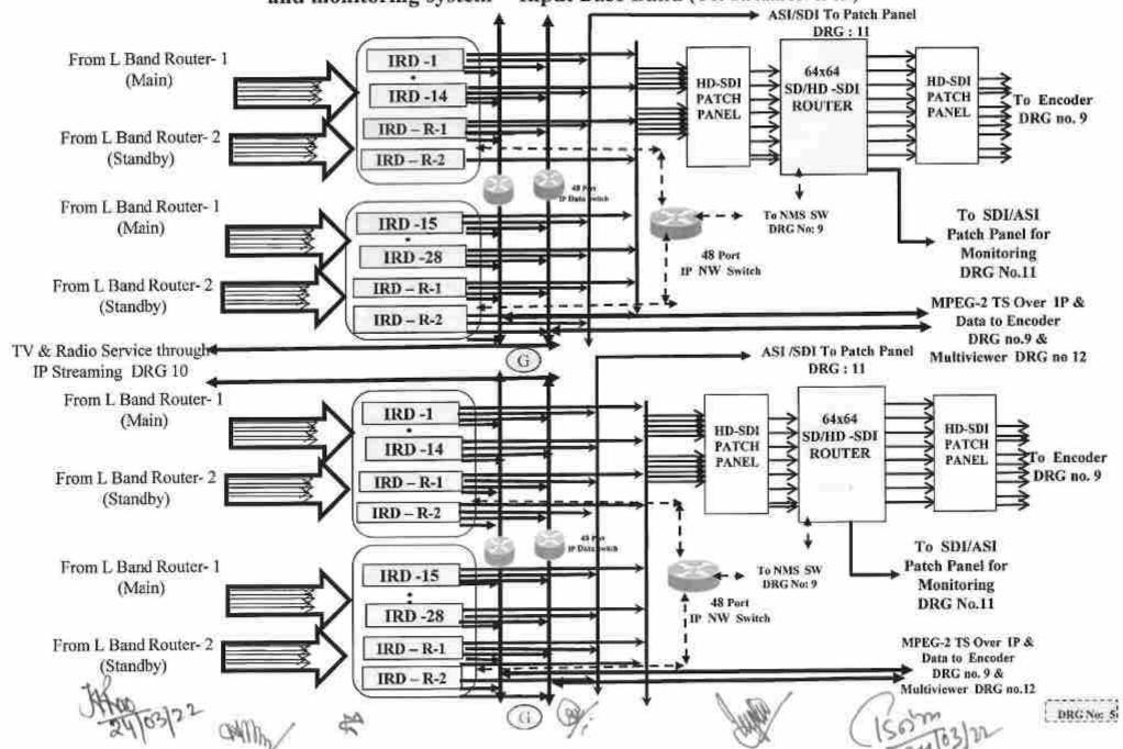
Suggestive Block Schematic for SITC of DD DTH expansion by upgradation of existing four compression chain and monitoring system - Input Base Band-Radio Service (For Stream ,IN, 2N, 3N & 6N)
