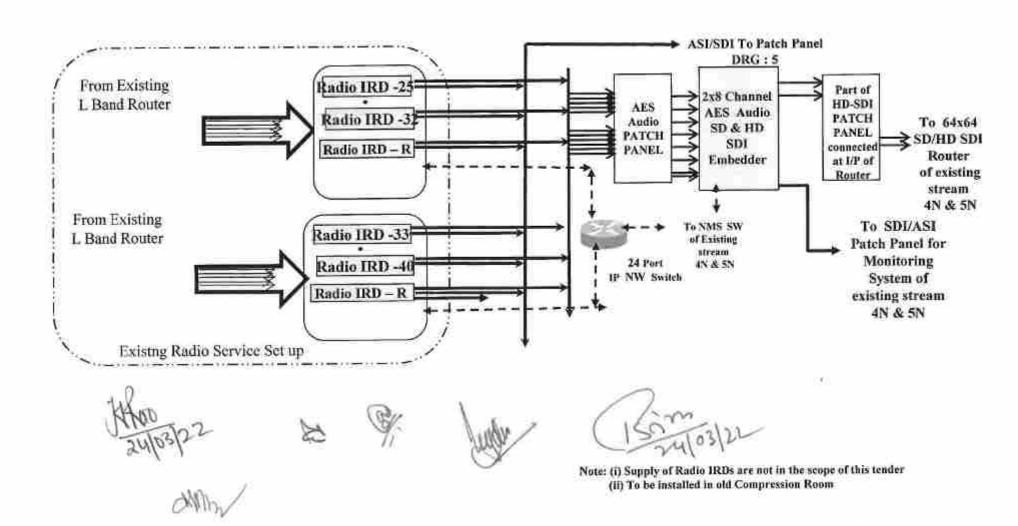
Suggestive Block Schematic for SITC of DD DTH expansion by upgradation of existing four compression chain and monitoring system Compression equipment for 1Nth Stream (Same for 2Nth Stream)
