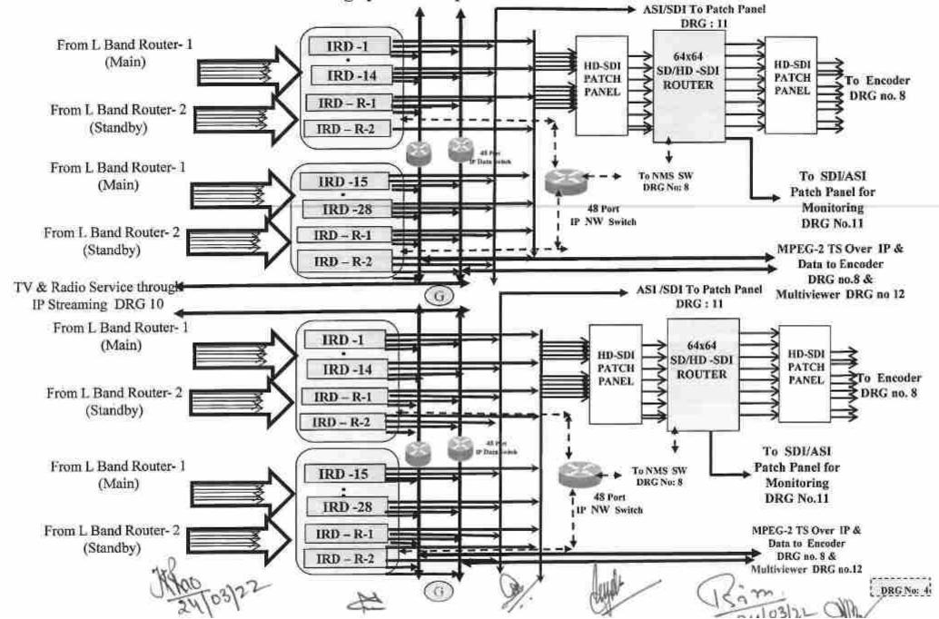
Suggestive Block Schematic for SITC of DD DTH expansion by upgradation of existing four compression chain and monitoring system - Input Base Band (For Stream 3N & 6N)
