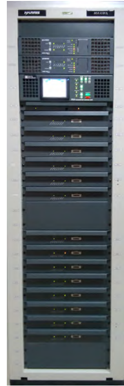
6kW DVB-T2 Transmitter
