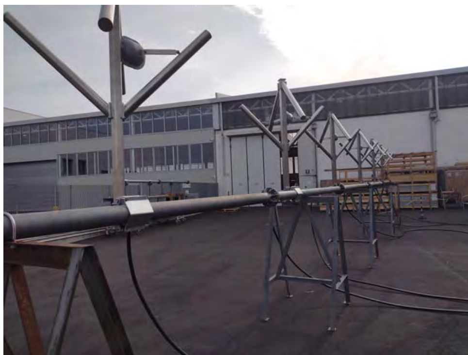
Phases and Amplitude - VSWR test of Antenna Systems
