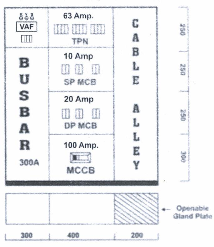
Notes :-All Dimensions are in MM cable Entry from Bottom and Top Fabricated with 18 G: CRCA Sheet Powder Coated Siemens Grey
