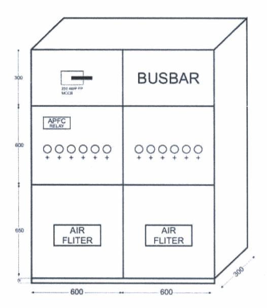
Notes :-All Dimensions are in MM. Febricated With 18G. CRCA Sheet Powder Coated Siemens Grey
